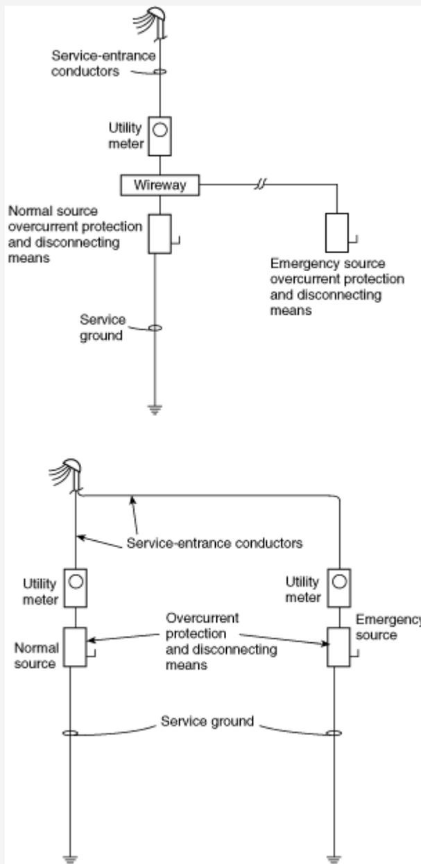
The advantage of connecting the emergency lighting circuit to the main power line on the live side of the main disconnect is service continuity if the main switch is thrown by employees or fire fighters as a precautionary measure. The *Code* does not prohibit this practice; however, it should be noted that this method does not meet the requirements for emergency lighting.
